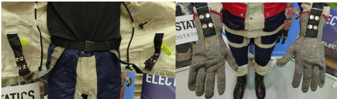
Figure 7 – Example of training demonstration on adequate bonding between conductive suit components
