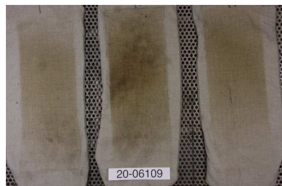
Fig. 1a, 1b – Examples of conductive fabric samples exposed to a vertical flame test
