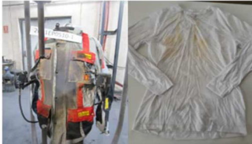
Fig. 2 – Example of a conductive garment arc test per ASTM F2621
