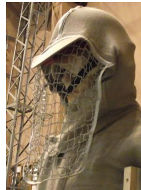
Figure 5. Additional face mesh installed on an existing type of conductive clothing (originally made without any face screen)
