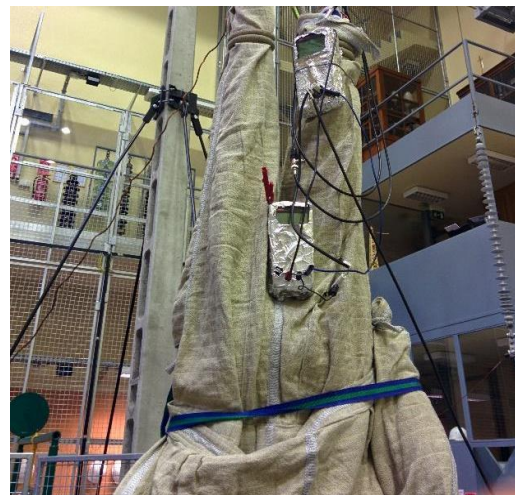
Figure 2. Inaccurate and dangerous way to measure leakage current by “shielded” micro-ammeters
